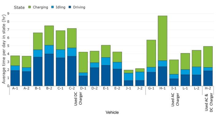
Compared to Q2 (the equivalent quarter in 2022), slightly more time was spent charging using AC chargers than driving, whereas less time was spent charging with DC chargers than driving.
