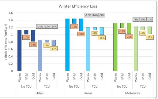
The apparent lesser impact of cold weather on vehicles with a TCU is mostly due to the summer efficiency of TCU vehicles being especially lower than that of non-TCU vehicles. As explained in subsequent slides, this is due to the TCU vehicles having an inherently lower efficiency overall due to their greater weight.
