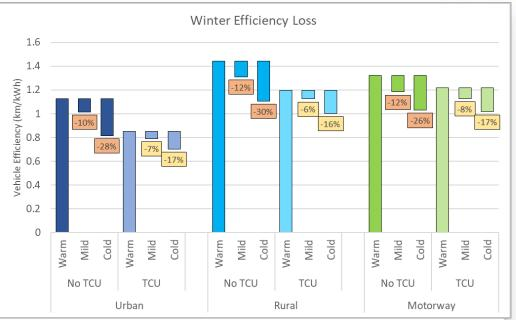
The vehicles with a TCU see a smaller 7% and 17% reduction across all drive cycles in mild and cold conditions respectively, compared to TCU vehicles in warm weather, as shown in the yellow boxes.
