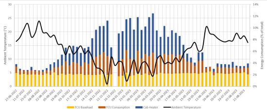
This raises the question: why is the efficiency of temperaturecontrolled vehicles especially lower in warmer summer weather compared to normal vehicles, as shown by the grey boxes on the previous slide? This seems counter-intuitive when the majority of ancillary consumption is in the winter.
