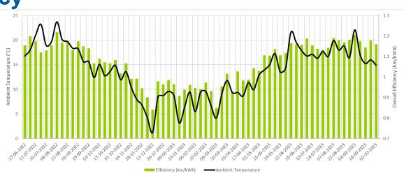
This graph includes all vehicles and ancillary consumption across all types of driving. The following pages dig down to see how the efficiency varies by drive cycle and ancillary consumption.
