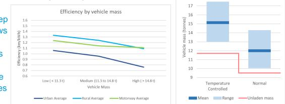
Due to including lots of start-stop activity, the efficiency of the urban drive cycle is especially lower for heavier vehicles.
