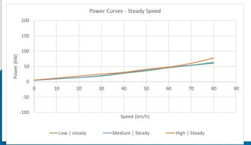
We would not expect the power requirement to vary much because at a steady speed on a flat road power is mostly required to overcome air resistance. Indeed, the power requirements are similar regardless of the payload.
