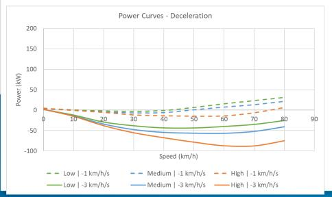
At 1 km/h/s regeneration is negligible, and due to air resistance at higher speeds power still needs to be applied even during gentle deceleration.
