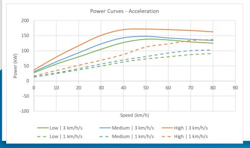
At moderate acceleration of 1 km/h/s it can take an additional 30 to 50 kW to accelerate above 50 km/h with a high payload compared to a low payload.
